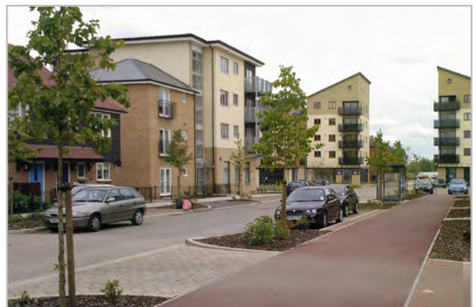
Primary streets that are bus routes should generally be straight and feel like more significant streets
