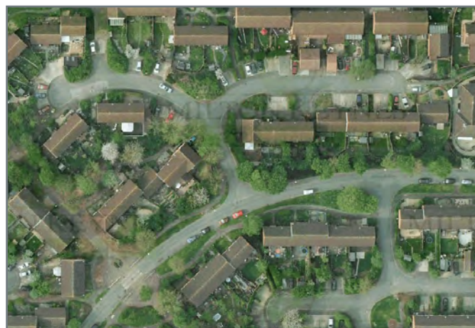
Florin Close, Leopard Drive, Noble Close in Pennyland - buildings positioned to capture solar gain
