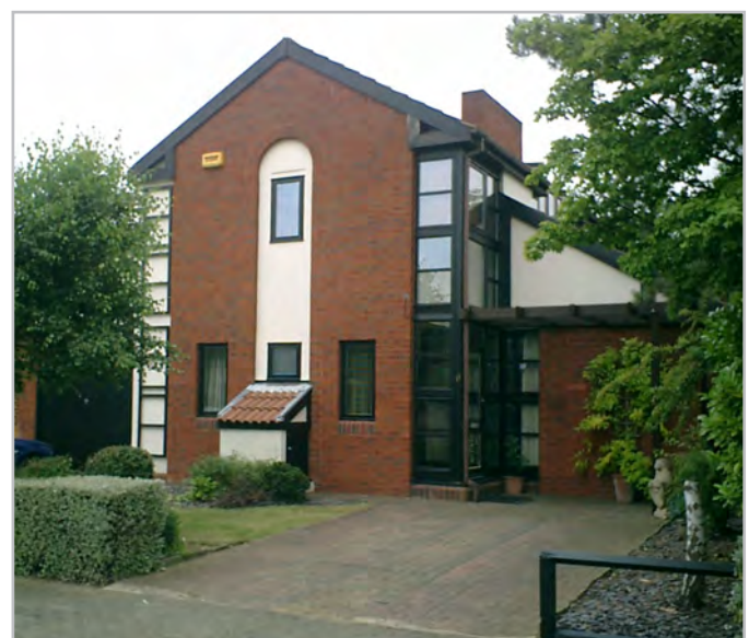
Larger setbacks allow for on plot parking and a softer edge to the street.
