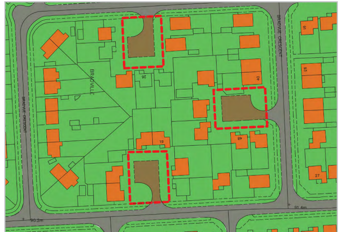
Culs-de-sac have been used to break up a larger block of approx 110m x 110m in Bradville
