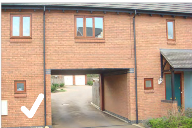
"Bridge over unit" makes a clearer definition that the rear court is private
