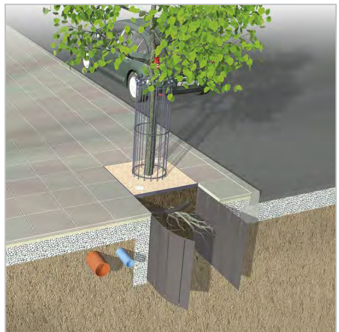
Root protection barrier detail
